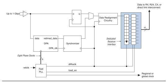
Figure 2-59. Stratix II Receiver Channel
