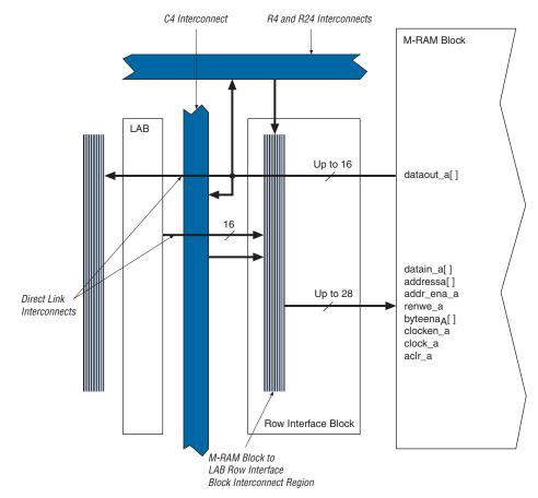
Figure 2-26. M-RAM Row Unit Interface to Interconnect
