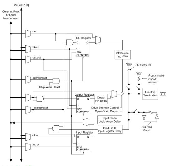
Figure 2–51 shows the IOE in bidirectional configuration.
