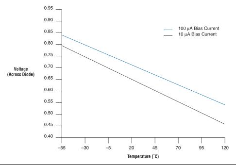
Figure 3–2. Temperature vs. Temperature-Sensing Diode Voltage
