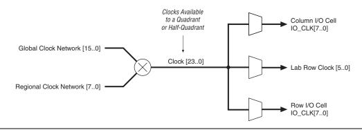
IOE clocks have row and column block regions that are clocked by eight I/O clock signals chosen from the 24 quadrant clock resources. Figures 2–35 and 2–36 show the quadrant relationship to the I/O clock regions.
