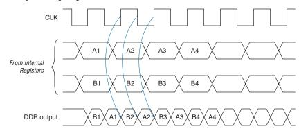
Figure 2-55. Output Timing Diagram in DDR Mode
