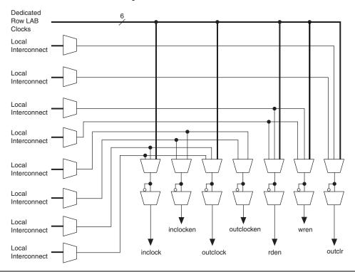
Figure 2-19. M512 RAM Block Control Signals
