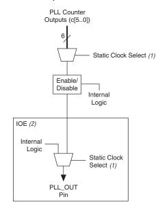
Figure 2–39. External PLL Output Clock Control Blocks
