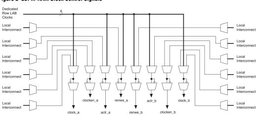
Figure 2-23. M-RAM Block Control Signals
