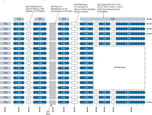
Figure 2-1. Stratix II Block Diagram
