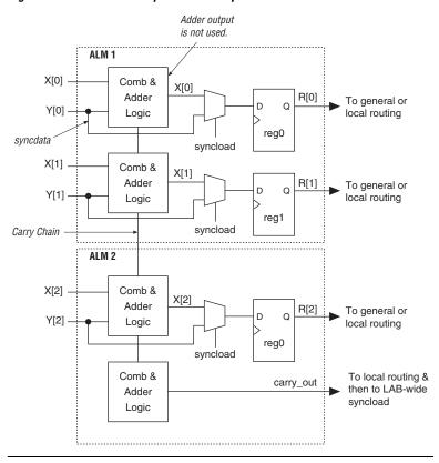
Figure 2-12. Conditional Operation Example
