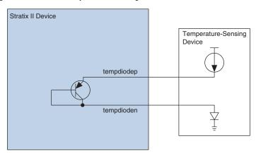
Figure 3-1. External Temperature-Sensing Diode
