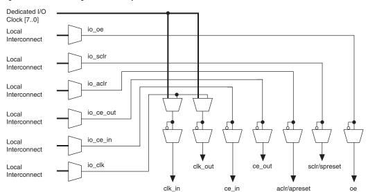
Figure 2-50. Control Signal Selection per IOE
