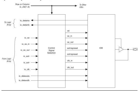
Figure 2-49. Signal Path through the I/O Block
