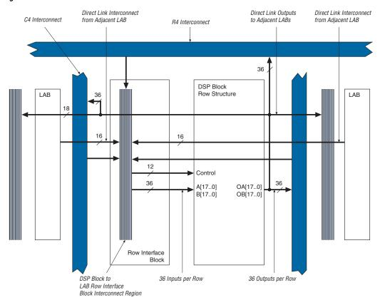
Figure 2-30. DSP Block Interface to Interconnect
