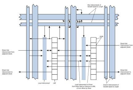
Figure 2-2. Stratix II LAB Structure
