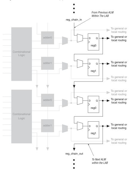
Figure 2–15. Register Chain within an LAB Note (1)
