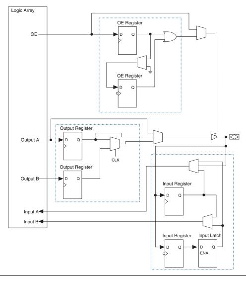
Figure 2-46. Stratix II IOE Structure
