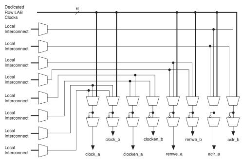
Figure 2-21. M4K RAM Block Control Signals
