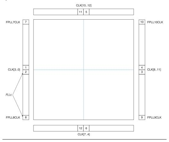
Figures 2–41 and 2–42 shows the global and regional clocking from the fast PLL outputs and the side clock pins.
