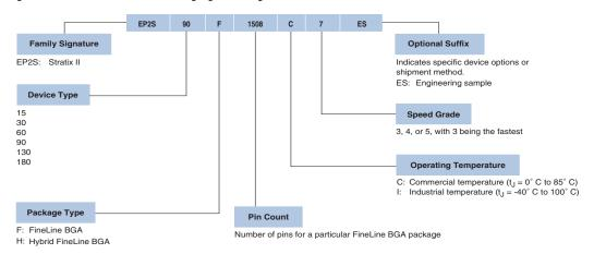
Figure 6-1. Stratix II Device Packaging Ordering Information
