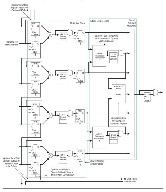
Figure 2-28. DSP Block Diagram for 18 x 18-Bit Configuration
