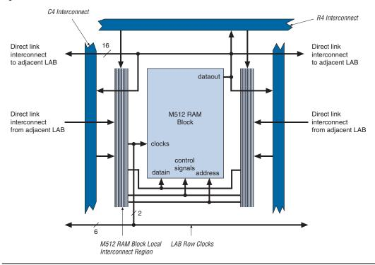
Figure 2-20. M512 RAM Block LAB Row Interface
