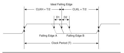
DCD expressed in absolution derivation, for example, D1 or D2 in Figure 5–7, is clock-period independent. DCD can also be expressed as a percentage, and the percentage number is clock-period dependent. DCD as a percentage is defined as
