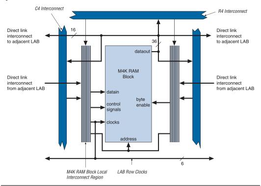
Figure 2-22. M4K RAM Block LAB Row Interface
