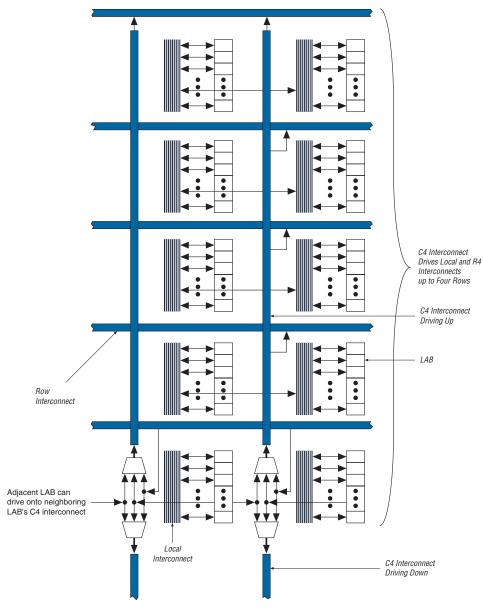
Figure 2–18. C4 Interconnect Connections Note (1)
